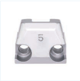
Die 5 For processing aluminium, mild steel and stainless steel 600 N/mm 2 up to 5 mm and stainless steel 800 N/mm 2 2.5 mm
